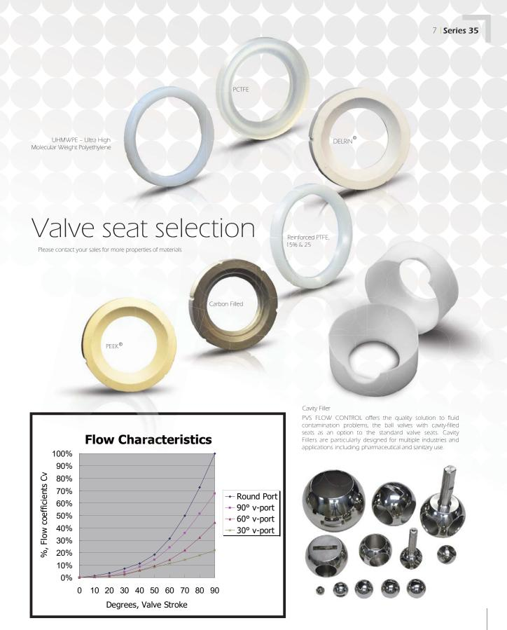
A v-port ball valve has a "v" shaped ball instead of a round-bore ball. This allows the orifice to be opened and closed in a more controlled manner with a closer to linear flow characteristic PVS FLOW CONTROL provides several v-port balls in Series 35 with different angles of "v". Note that the long-term throttling operation in a certain percent open is no recommended. For Cv, please see Flow Coefficients (Cv) of V-port Ball Valve.
