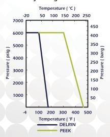
This table express Seat material resistance as declared by the original manufacturers. The values are to be considered with other parameters such as size, seat design and temperature limitations as governed by relevant standards such as ASME B16.34 or EN-12516.
